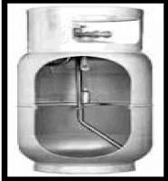
WARNING: Using a liquid withdrawal (fork truck) propane tank will clog the orifice in the heat tool and result in an extremely long and dangerous flame.
