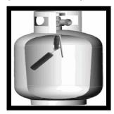
B. Not Correct: Liquid withdrawal—Do not use this style (used on fork trucks)
