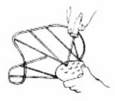
5.3 Attach the guard assembly to the combustor (30) with the 4 mounting screws (41).
