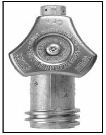
To open the flow of propane, turn the tank hand wheel in a counter clockwise motion and watch the regulator gauge increase to the required 22 PSI.
