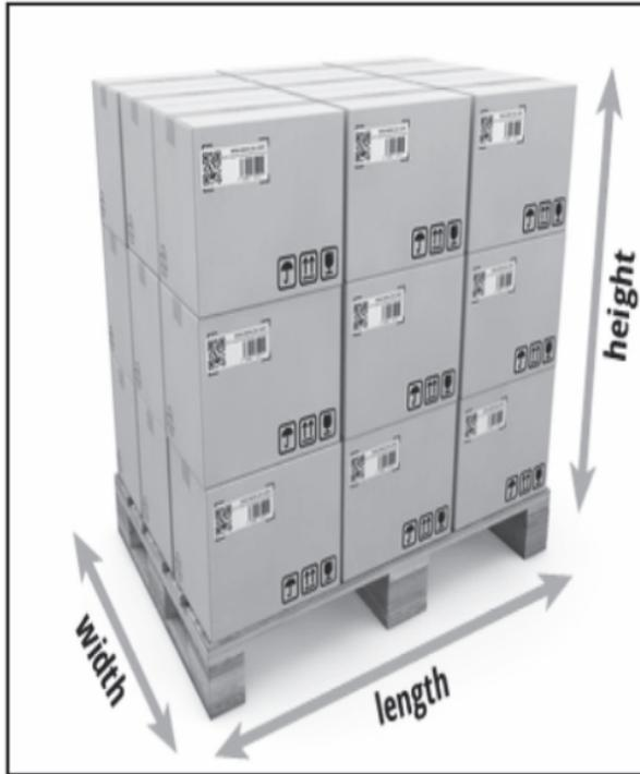
1) Measure the length, width and height of the pallet to be covered.
