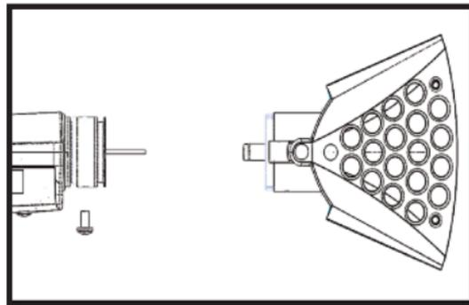
*Remove # 16 Combustor Assembly*
